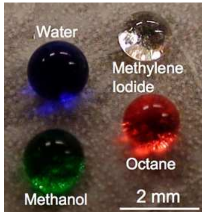
Figure 2.11: Photos of water (colored blue with methylene blue) (72.2 mN/m), methylene iodide (50.0 mN/m), methanol (colored green) (22.7 mN/m) and octane droplets (colored red with oil red O) (21.6 mN/m) on a lotus leaf surface covered with electrospun fibers (beads-on-strings morphology) of PMMA (polymethyl methacrylate) + 44wt% fluorodecyl POSS (polyhedral oligomeric silsesquioxane molecules). (71)(72)
