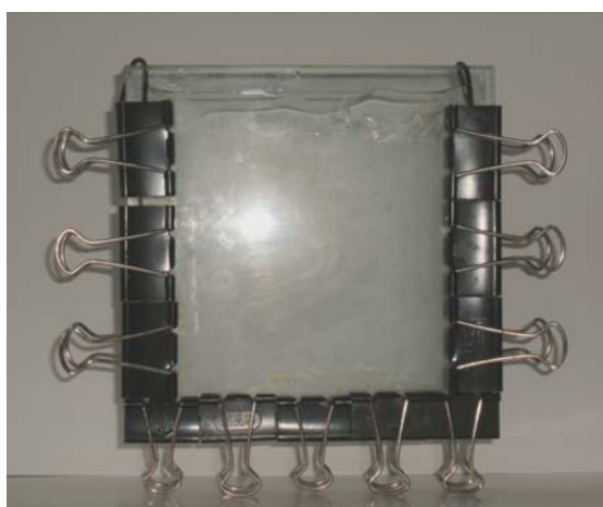
Figure III.1. A glass mold used for the preparation of thermosensitive hydrogel films
