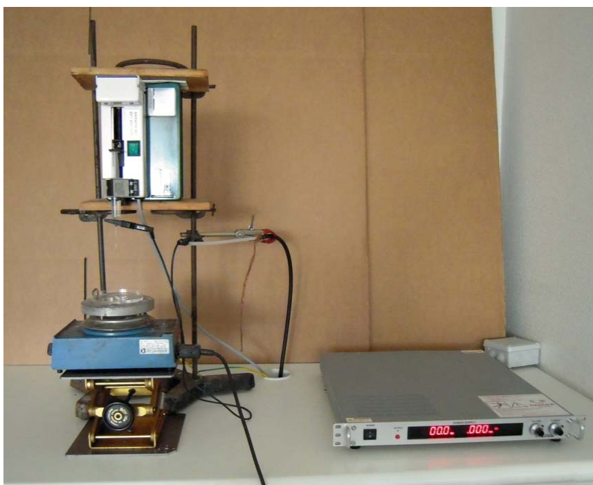
Figure II.10. Laboratory setup for the electrostatic extrusion
