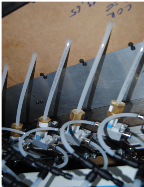
Figure 4.8: Actuators installed on the interchangeable plates
