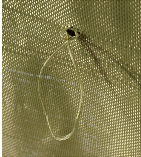
FIGURE 2.7 – Arrachement d’un fil
