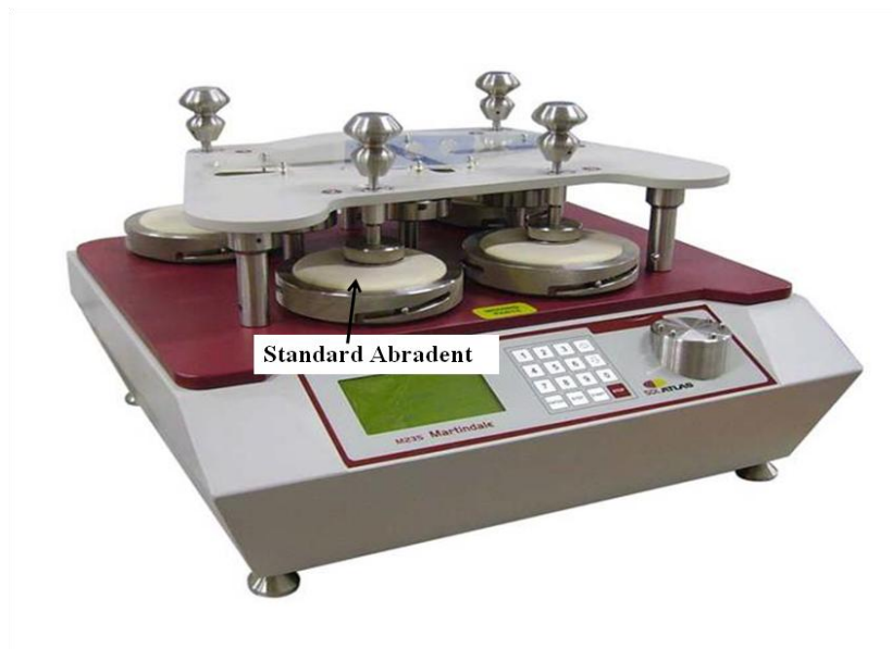
Figure 16: M235 Martindale Abrasion Tester used for rubbing durability test
