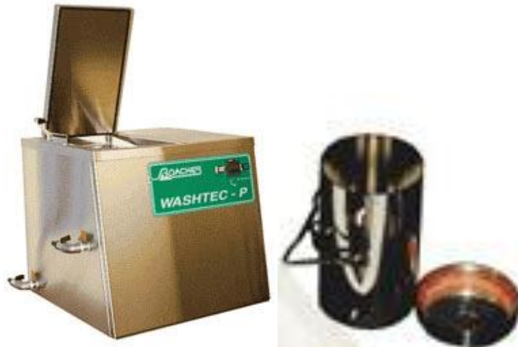
Figure 15: Washtech-P machine used for water durability test and washpot
