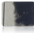
Figure 3- 5- Glass Substrate with Zn Seed Layer by thermal evaporation in vertical furnace: the black zone presented the zone with the deposited Zinc film.
