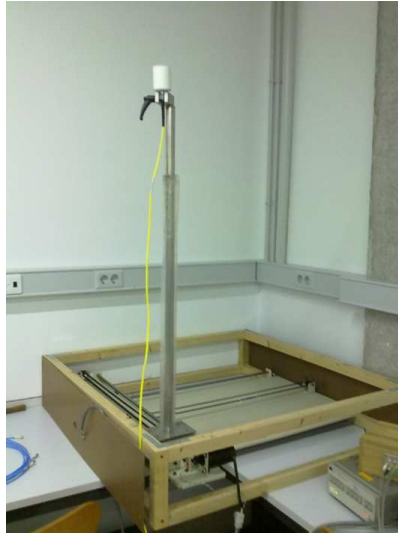
Figure 2.8. XY positioning board with the transmitting antenna.
