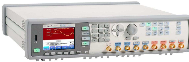
Figure 2.29. Base band signal generator.
