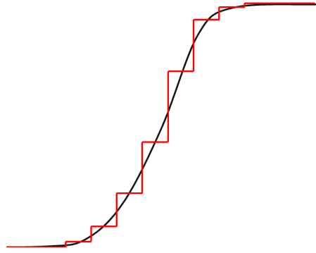
Figure 3.10: Decomposition of a non-homogeneous optical index profile into homogeneous films
