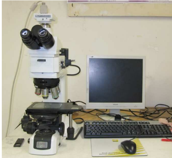
Fig. 6.12. View of optical microscope Nikon Eclipse LV100 set up.
