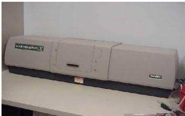
Fig. 6.2. View of Malvern Mastersizer X particle size device [61].
