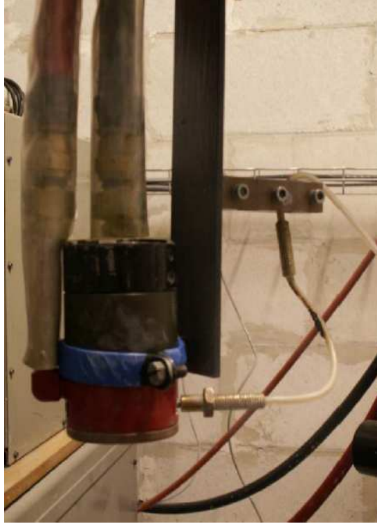
Fig. 6.9. View of set up of internal mode with the use of continuous jet nozzle injector installed inside the plasma torch [56].
