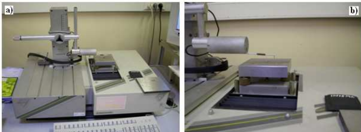
Fig. 6.13. Somicronic ST-11a instrument (a), and working table with measuring head (b).
