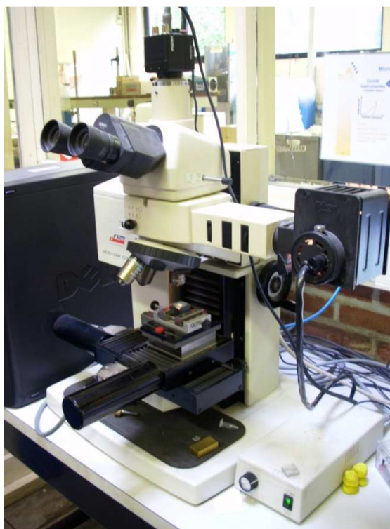
Fig. 6.15. CSM+ instrument for scratch test investigations.
