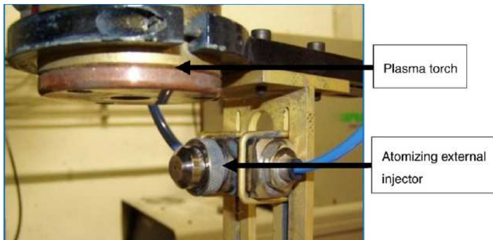
Fig. 7.12. Set up of the suspension injector – external atomizing mode [4.9].
