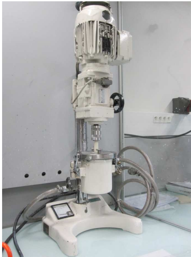
Fig. 6.1. View of attrition milling device moliNEx system (NETZSCH).
