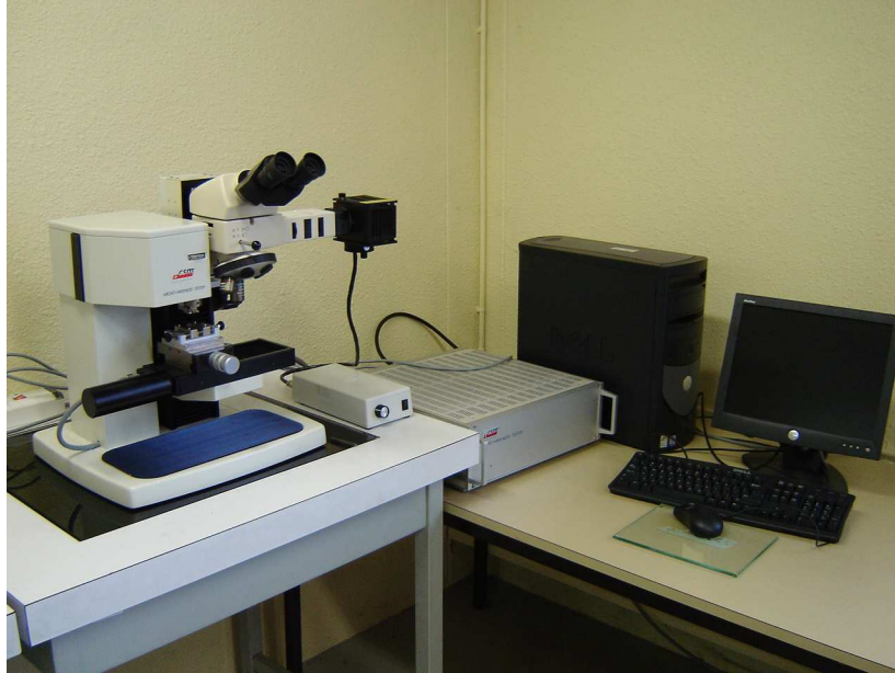
Fig. 6.17. Microhardness tester CSM 2-107 equipped with Vickers indenter.
