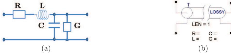
Figure 2-30 Transmission line (a) lumped circuit (b) TLOSSY element
