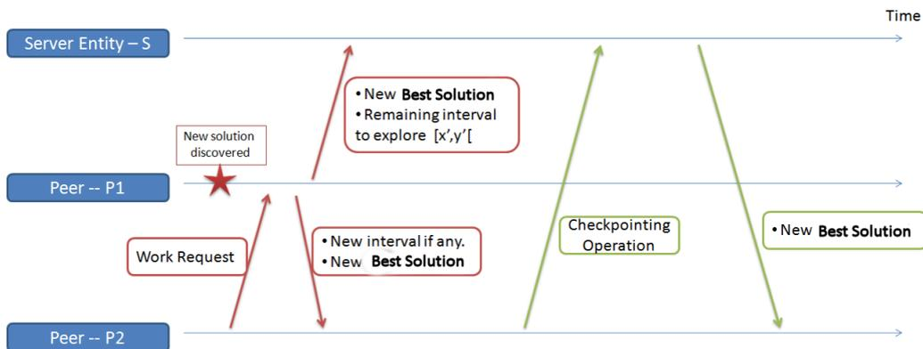
Figure 6.8: Sequence diagram representing the Best Solution Sharing mechanism.
