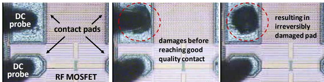
Fig. 2.18 – Illustration of the effect of a thick and soft material below the micrometer scale metallization of a thinned sample transferred onto a 3M adhesive film: (from left to right) a DC probe is slightly contacted to the ground aluminium pad, the contact quality is however not sufficient to characterize the device, and the contact pad is irreversibly damaged before achieving a good contact.
