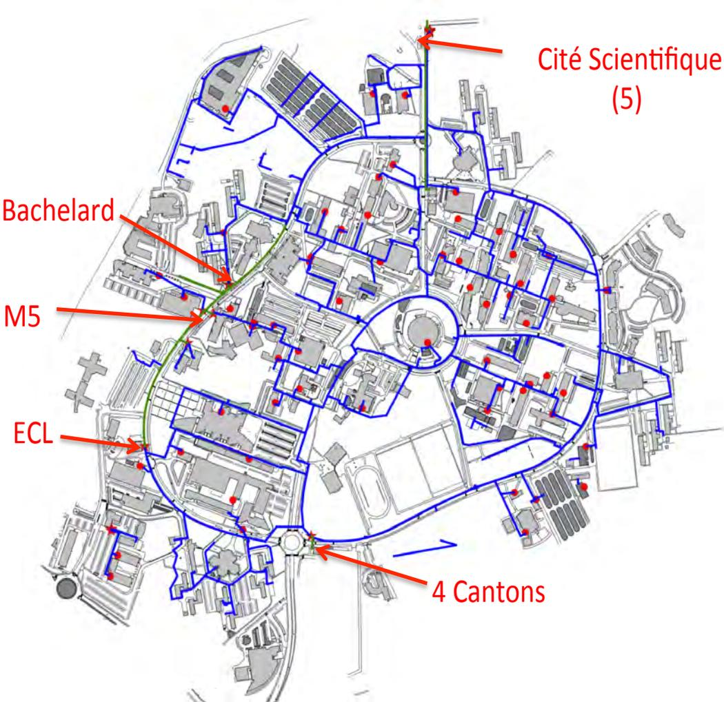
Figure 2.4 Water supply net work of the Scientific Campus
