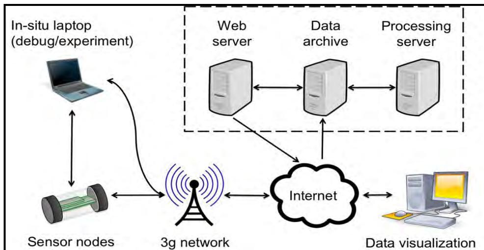
Figure 1.11 Communication system used in Singapore Project
