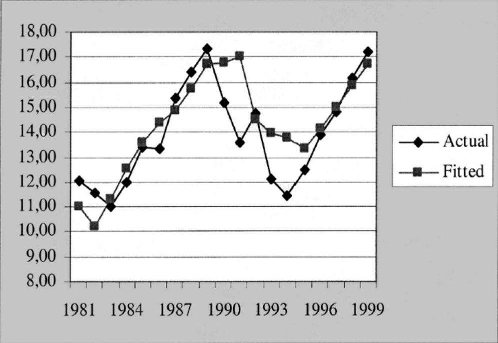
Figure 1.1 Simulation of the residential water consumption in the City of Athens (Bithas and Stoforos, 2006)
