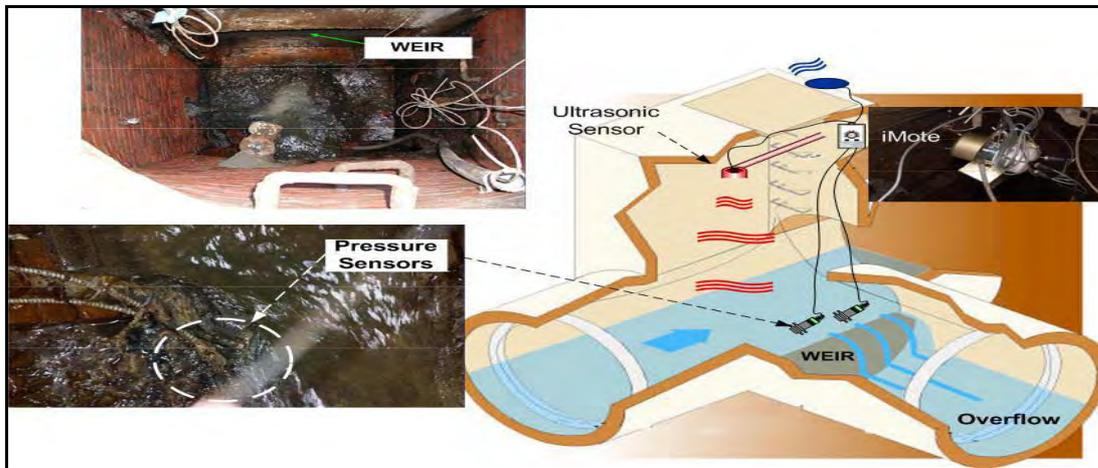
Water level Monitoring in the sewer outflow collector
