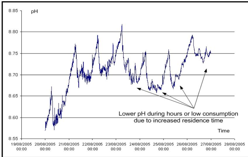
**Fig 1.8 pH record (Boston Smart Water System)**
