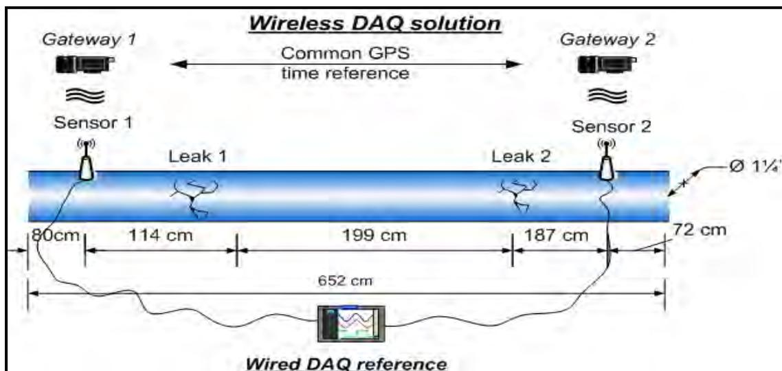
*Fig 1.7 Laboratory pipe rig for the water leakage detection in Boston*
