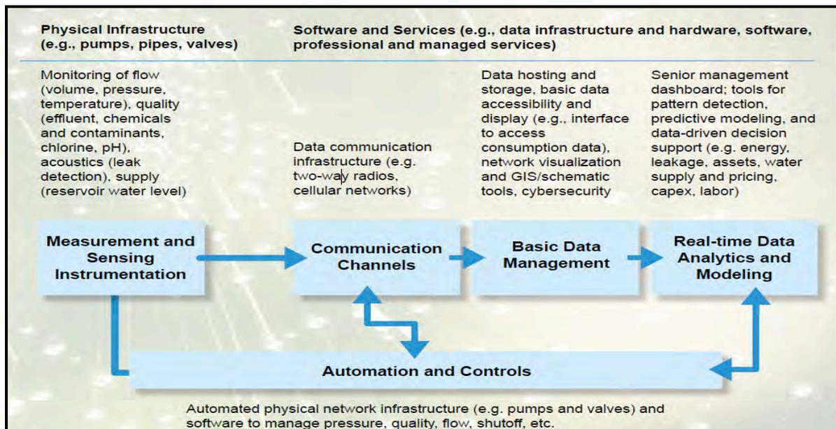
**Figure 1.4 Layers of smart water network**
