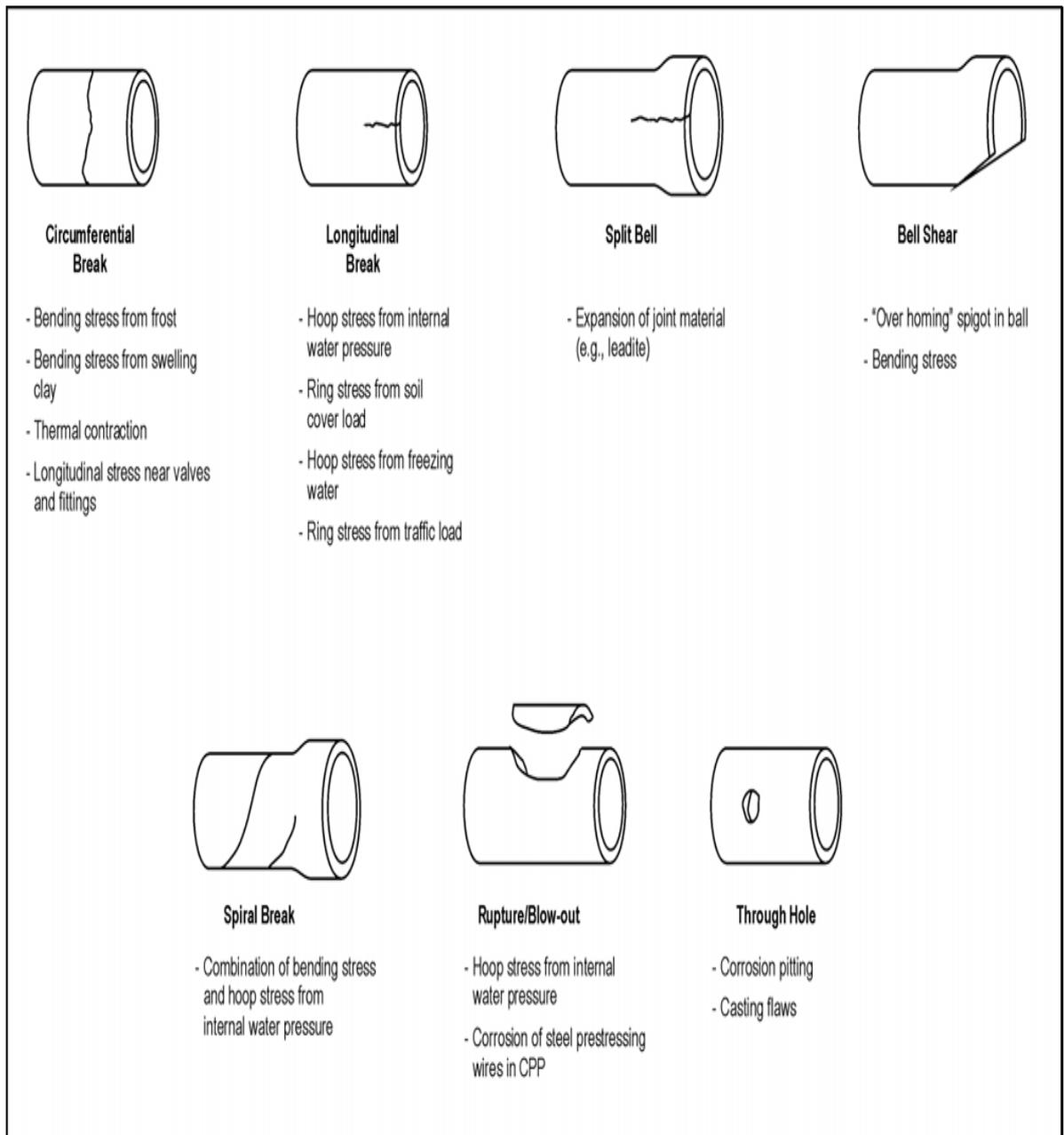
**Figure 1.2 Modes of failure in water mains**
