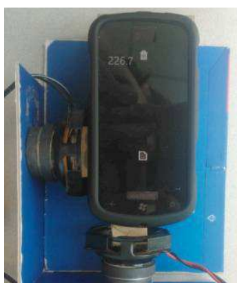
Figure 2.34 The two actuators produced lateral movement of the mobile phone (adapted from [87]).
