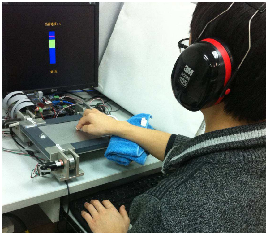
Figure 5.4 Experiment setup for both experiments. In the training session of the second experiment, a slider was shown on the computer monitor to represent the normal force. Participants were instructed to maintain the normal force in the green area which indicated the gauge output of 1-1.5 N. The slider was hidden when the experiment started.
