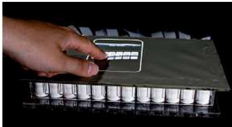
Figure 2.35 MudPad is a system that provides localized haptic feedback independently at multiple points (adapted from [88]).
