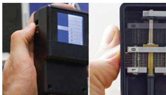
Figure 2.6 The tactile transducer used in a handheld device to provide lateral traction on the surface of the finger skin (adapted from [47]).
