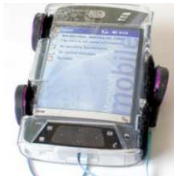
Figure 2.13 The multi-actuator PDA used to indicate downloads progress (adapted from [60]).
