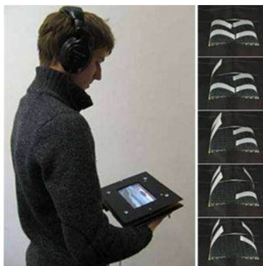
Figure 2.36 The user holds the mobile TV and feels haptic feedback at the back of the device. The ultrasonic acoustic pressure moved tapes when various regions of transducers are triggered (adapted from [89]).
