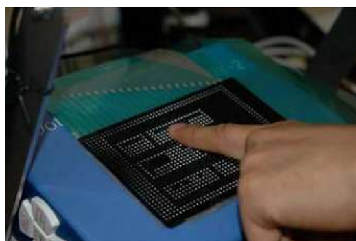
Figure 2.25 Displaying text and pictures using pins (adapted from [76]).
