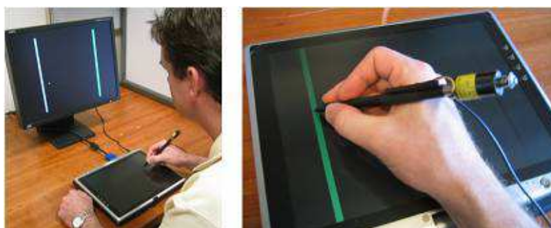
Figure 2.17 Indirect and direct input with a Haptic Pen (adapted from [13]).
