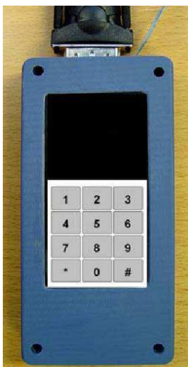
Figure 2.20 The “Snap-Crackle-Pop” tactile mobile device (adapted from [64]).
