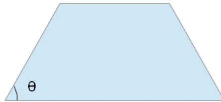
Figure 27 Schematic view of NCs with same diameter of 704 nm for a given period of 880 nm and length of 350 nm. \theta is the angle between lateral sides and bottom.
