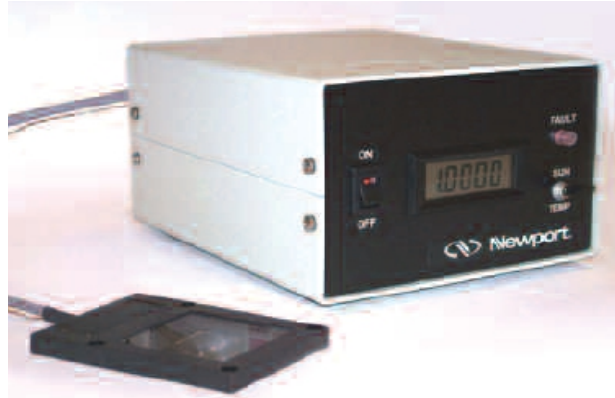
Figure 23 Photograph of reference cell and electronic display
