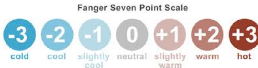
Fig. 1.7 Values of PMV according to Fanger
