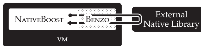
Figure 3.7: NATIVEBOOST generates native code at language-side with BENZO to perform an FFI callout to an external function.
