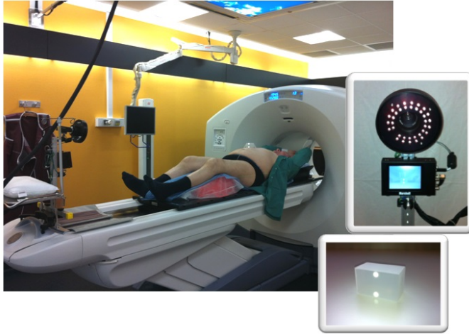
Figure 2.11: Patient examination with the Real-Time Position Management System (RPM) - infrared camera and reflective box
