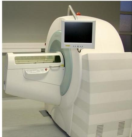
Fig 2-7 :  $\mu$ CT/ $\mu$ PET-scanner Inveon Siemens.
