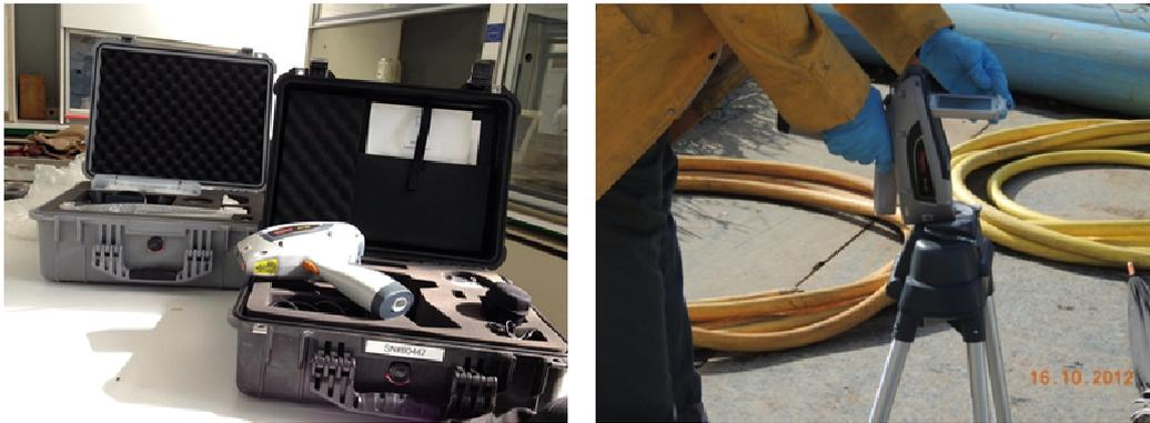
*Figure 2.8: mobile unit X-ray fluorescence*
