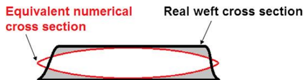
Figure 4.16: Lapeyronnie et al.'s model for layer to layer angle interlock, adaptation of the yarn cross section shape to lenticular with keeping constant area. (Lapeyronnie et al. 2011)
