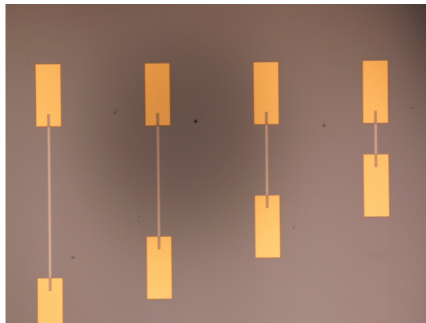
Figure 2.21: Photograph of Ti resistances with Au access pads taken with an optical microscope. The resistances shown are 8 \mu\text{m} wide and between 100 \mu\text{m} and 486 \mu\text{m} long.
