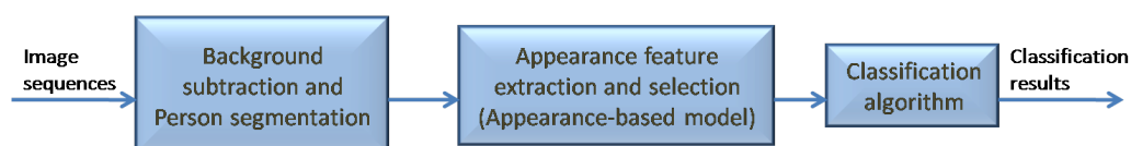
Figure 4.16: General architecture of appearance-based human recognition system
