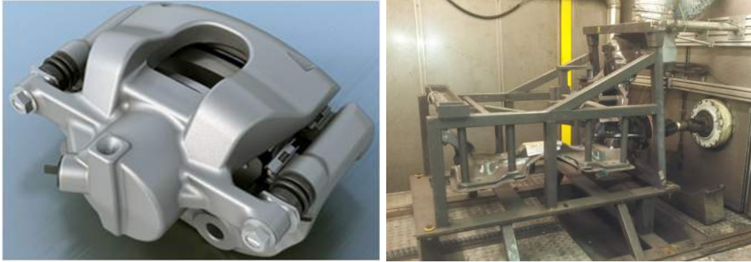
Figure 2.26: Floating caliper brake adapted on an inertia dynamometer bench
