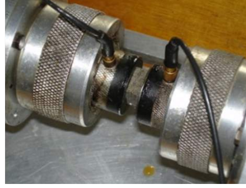
Figure 2.20: Ultrasonic testing transmission setup
