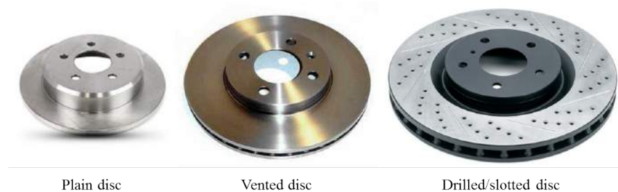
Figure 1.2: Types of disc brake
