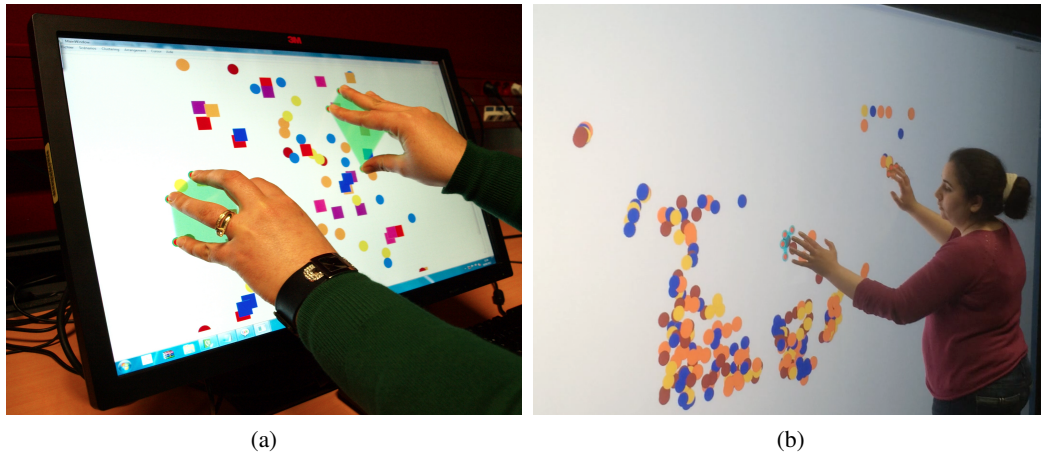
Figure 7.6: Two simultaneous rigid movement induced by one user using two hands on a 3M screen (a) and a large screen measuring 4 x 2 meters (b).
