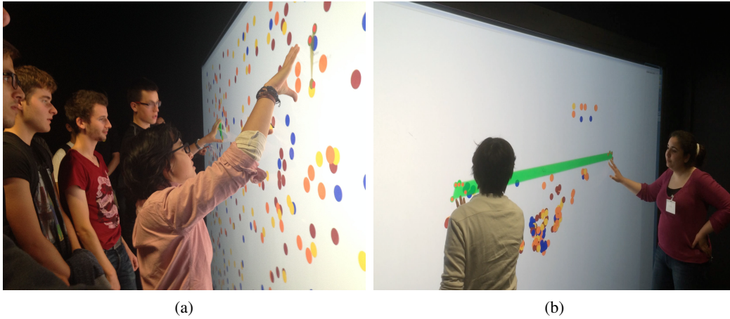
Figure 7.7: Examples of deploying our technique on a large interactive surface ( 4 \times 2 meters): three users performing three independent simultaneous rigid movements (a) and two users collaborating to form the same rigid movement (b).
