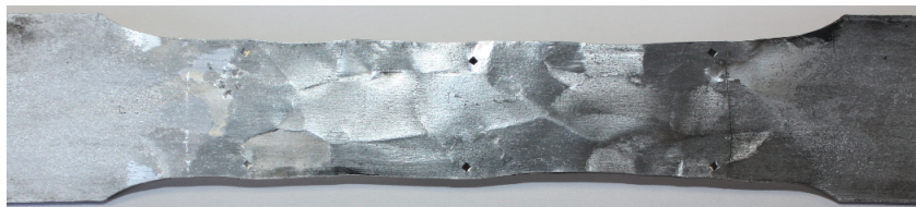
Figure A.6: The deformed specimen after a tensile test
