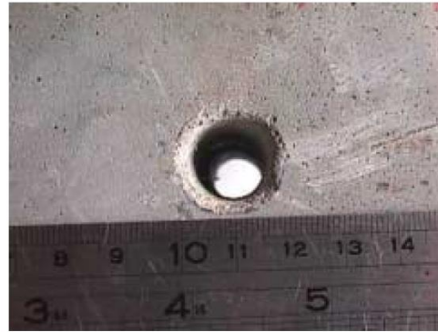
Figure 1.22: Scheme of the microwave drilling apparatus and configured hole (Jerby and Dikhtyar, 2001)
