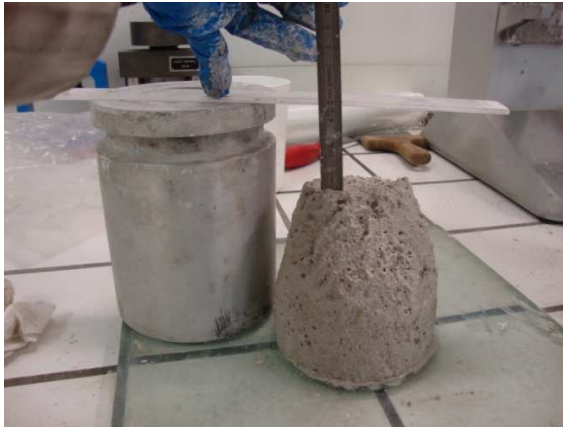
Figure 4-3 Cone MEB used for measuring slump of mortar (In the right figure the unit is mm)
