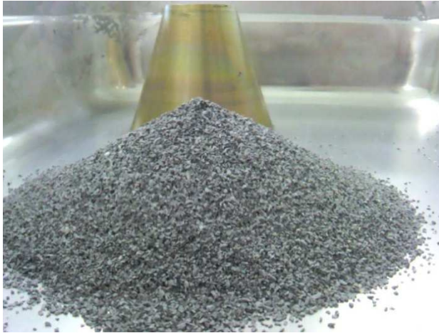
Figure 2-4 Shape of cone corresponding to the SSD state (EN 1097-6 method)
