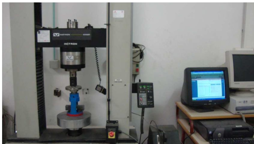
Figure 4-4 INSTRON machine used for mechanical testing of mortars
