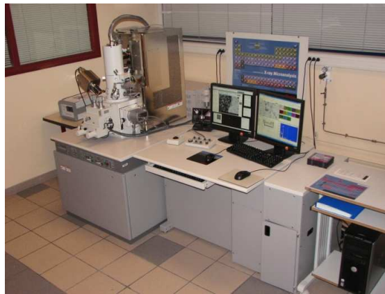
Figure 4-5 SEM with EDS analysis used by the HITACHI S-4300 SE/N
