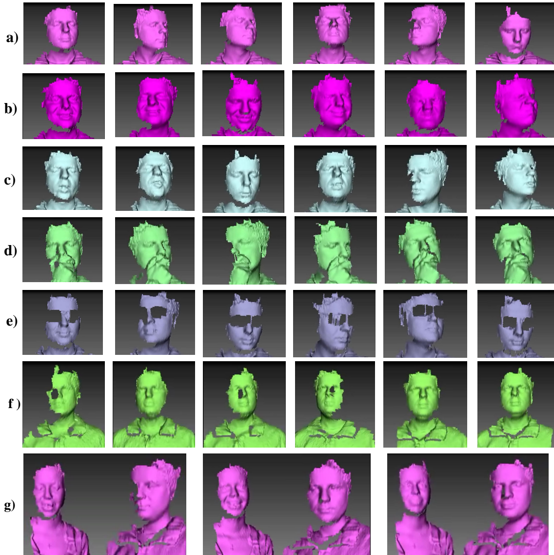
Figure 4.11: The 3D dynamic sequences acquired under different conditions: a) neutral; b) expressive; c) talking; d) internal occlusion by hand; e) external occlusion by sunglasses; f) walking and g) multiple persons.
