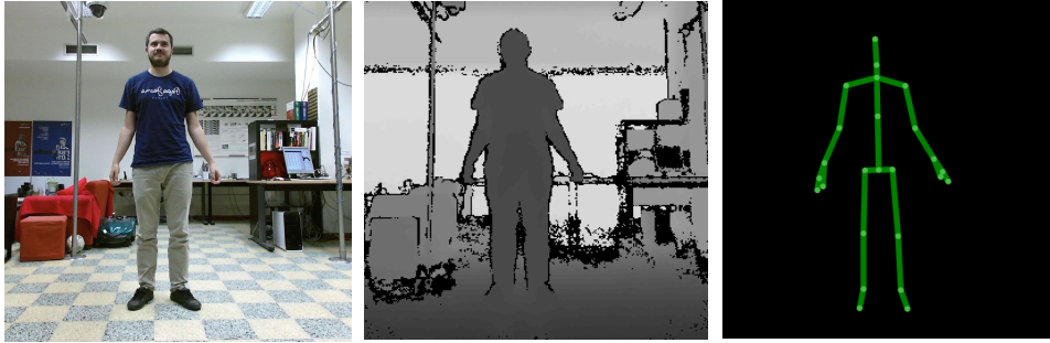
Figure 2.4 – Example of data provided by RGB-D sensors like Microsoft Kinect 2: 2D color image (left), depth map (middle) and 3D skeleton (right).
