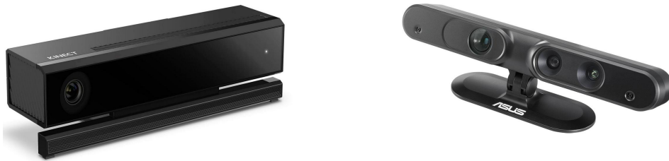
Figure 2.2 – Example of RGB-D sensors. Left: Microsoft Kinect 2 [56]; Right: Asus Xtion PRO LIVE [7].
