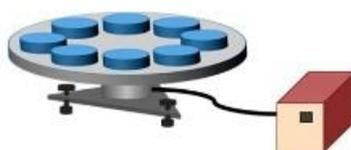
**Figure 20.14.** Schema of the evaporative dish method setup
