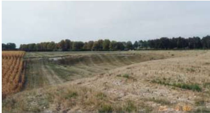
Figure 1.15. Generalized subsidence on surface over a chalk quarry at Indre et Loire, France - Document by INERIS
