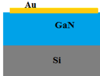
Figure 4.37. Top electrode configuration: Argon etching and evaporation-Au 40 nm on GaN/Si thin film
