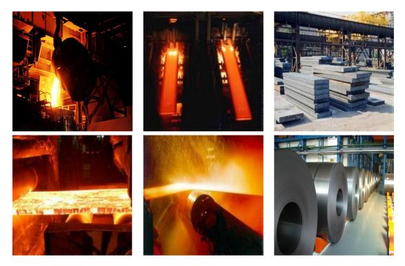
Figure 1.1: Quick overview of the steel making process, from hot liquid metal to coils.
