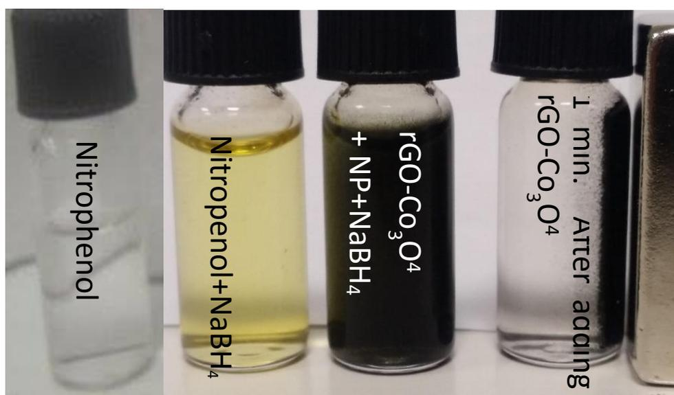
**Figure 4.17:** Photograph images of the catalytic reduction of 4-NP to 4-AP using rGO-Co<sub>3</sub>O<sub>4</sub> nanocomposite as catalyst and its separation at the end of the process using a magnet.
