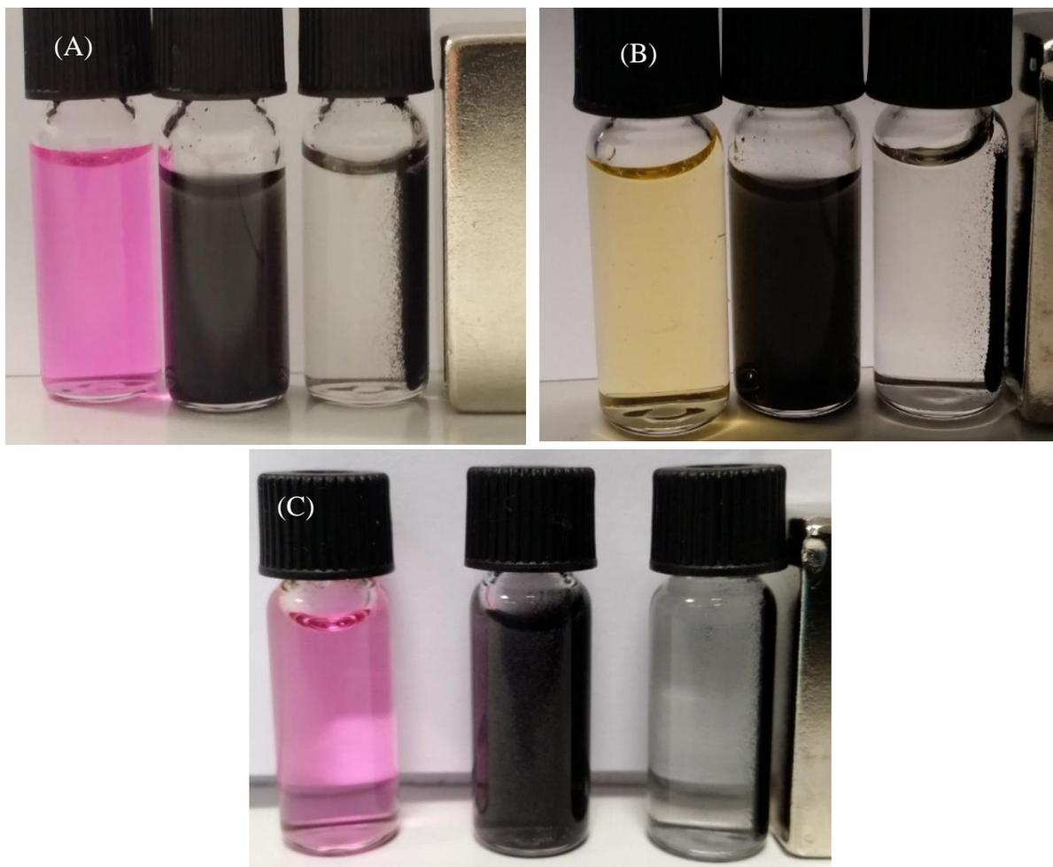
**Figure 4.33:** Photographs of (A) RhB, (B) MO and (C) Rose Bengal aqueous solutions before and after treatment with 1 mg/ml of rGO-Co<sub>3</sub>O<sub>4</sub> nanocomposite. The right photos correspond to the solutions of the bottles in the centre upon application of an external magnet (1 Tesla).
