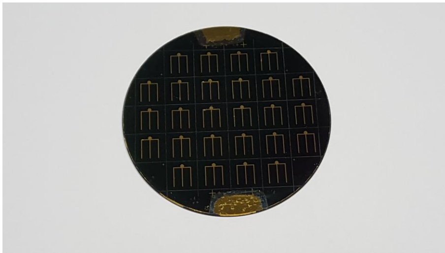
Figure 5.1: Final view of a 2" wafer on which 26 0.5cm 2 cells have been defined. The gilded zones that are visible at bottom and top correspond to back electrode contacting areas.
