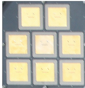
Figure 2.9: 8-element URA with dual-polarized slot patch antennas.
