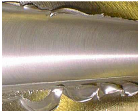
Figure I.27. Weld with a ribbon-flash defect. ( Mishra and Mahoney, 2007 )
