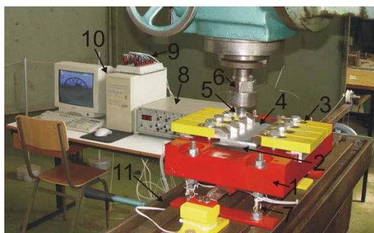
Figure I.14. Research site: 1 - The base plate, 2 - Support plate, 3 - Work piece clamp, 4 - Work piece of Al alloys, 5 - Tool for FSW, 6 - Clamp part of the milling machines, 7 - Special carrier with glued measuring tapes, 8 - Measuring bridge, 9 - BAS, 10 - PC with A/D card and software GLOBAL LAB, 11 - Work table of milling machine. ( Vukčević et al., 2011 )
