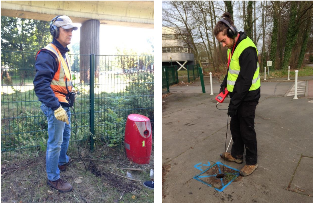
Figure 4.4: Leak detection operators with their electronically amplified sticks
