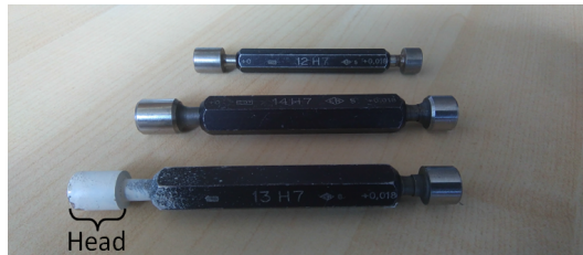
Figure 4.2: Painted plug-gage head to eliminate surface aspect problem.
