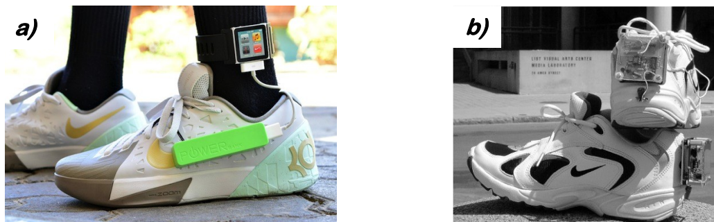
Fig. 2-5 a) Nike+® shoes for running with piezoelectric generator installed in shoe's heel, b) prototype shoes with piezoelectric harvester and RFID electronic circuit [Shenck, 2001]
