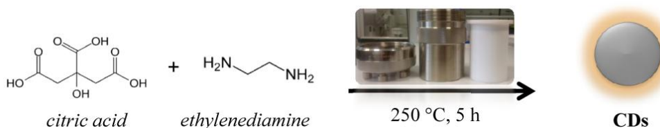
Figure 3.9. Schematic illustration of the amino-functionalized CDs synthesis.
