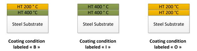
Figure II.2-5. Scheme of the heat treatment of every single electroless Ni-P coatings deposited on the steel substrate plates.
