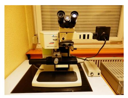
Figure II.3-1. Microhardness indenter CSM 2–107 manufactured by CSM instruments used to perform the instrumented indentation tests at the microscale range.
