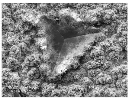
Figure I.2-2. SEM micrograph from the residual impression left by a Berkovich indenter on a hydroxyapatite coating sample.
