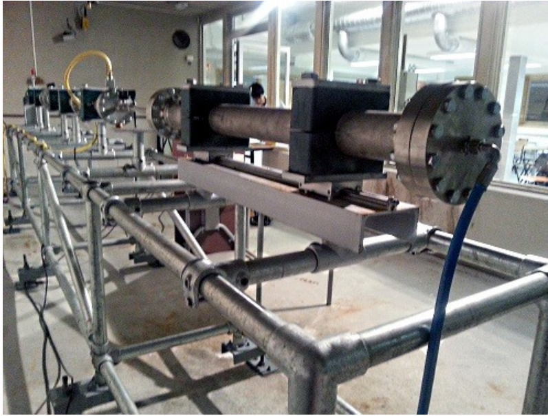
Figure 2.31 – The shock tube: Driver section to the right (containing compressed air) and driven section to the left containing uncompressed water and a T-section for mounting the test specimen.[66]
