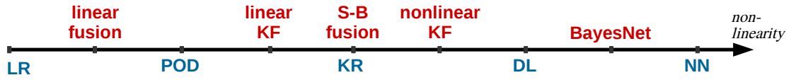
Figure 1.3 – Spectrum of models ordered by their level of nonlinearity (from left to right). Methods for mapping large-small scales are in blues, while those for fusion of measurements are in reds. Notations: linear regression (LR), proper orthogonal decomposition (POD), Kalman filter (KF), kernel regression (KR), similarity-based (S-B), dictionary learning (DL), Bayesian network (BayesNet), neural network (NN).
