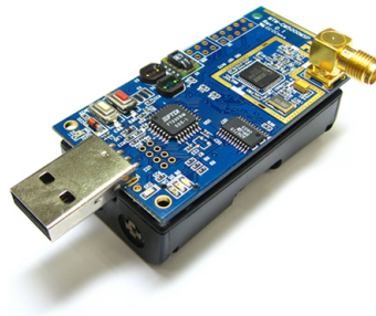
FIGURE 5.7: Maxfor sensor node. (source http://www.maxfor.co.kr )
