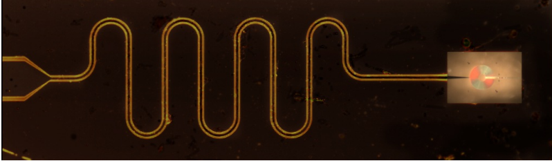
Figure 59. 70 \Omega quarter wavelength resonator and coil. The whole chip is 3 \times 10\text{mm}^2 .
