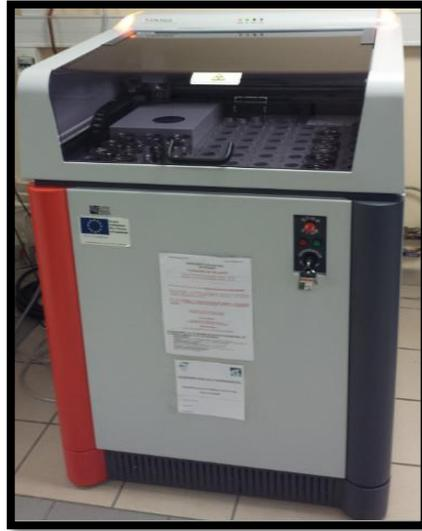
*Figure 22: Appareil de Fluorescence X (FX).*
