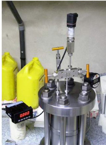
Figure 2.5: Gas breakthrough experiment with increasing upstream gas pressure [Duveau et al., 2011].
