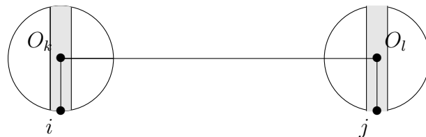
Figure 2.9: The black line is the distance between two points i and j which are located in two different clusters. The gray band is the concentration measure band.
